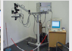
XRF ARTAX (Ø 100 µm, Ø 1 cm)
