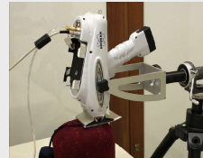
XRF Tracer (Ø 1 cm)
