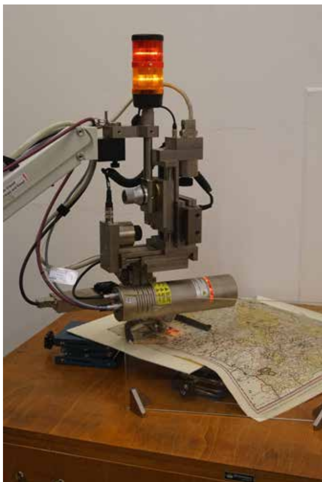
Fig. 1.2.7-1: Foto der Röntgenfluoreszenzanalyse (Safe SHWA). | Photo of the X-ray fluorescence analysis (Safe SHWA).
