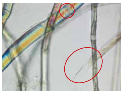
Fig. 20a: paper-mulberry fibres, cross-markings and a naturally rounded fibre end enveloped by a transparent membrane (red oval). Observed under the microscope at 400× magnification in manuscript DS 0062 00294 from the Buddhist Archives of Luang Prabang, Laos.
