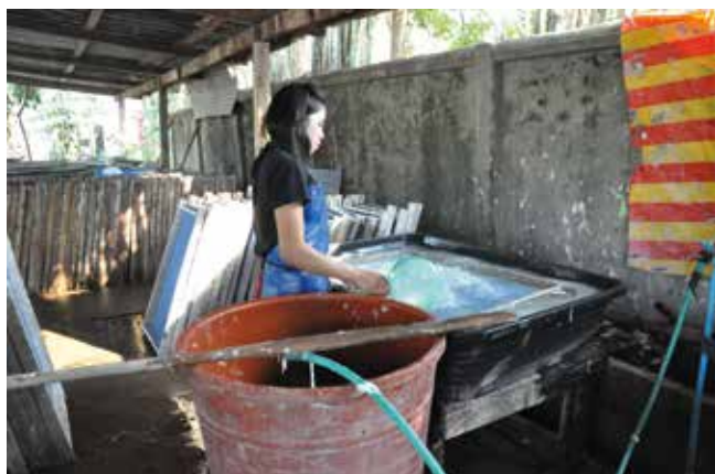
Figs 24a, b: The paper-sheet formation method using a fixed mould with a plastic screen attached to a wooden frame. Observed at Say Namkhan Company in Luang Prabang, Laos. The floating method is characterised by pouring paper pulp directly onto the sieve in carefully measured scoops (similar to a technique widely used in the Himalayas).
