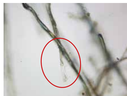
Fig. 20c: The natural fibre end enveloped by a transparent membrane, also with a natural round end, observed at 200× magnification in manuscript CMRU ARP.060 from the Chiang Mai Rajabhat University Library, Thailand.
