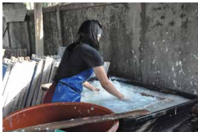
Figs 24a, b: The paper-sheet formation method using a fixed mould with a plastic screen attached to a wooden frame. Observed at Say Namkhan Company in Luang Prabang, Laos. The floating method is characterised by pouring paper pulp directly onto the sieve in carefully measured scoops (similar to a technique widely used in the Himalayas).
