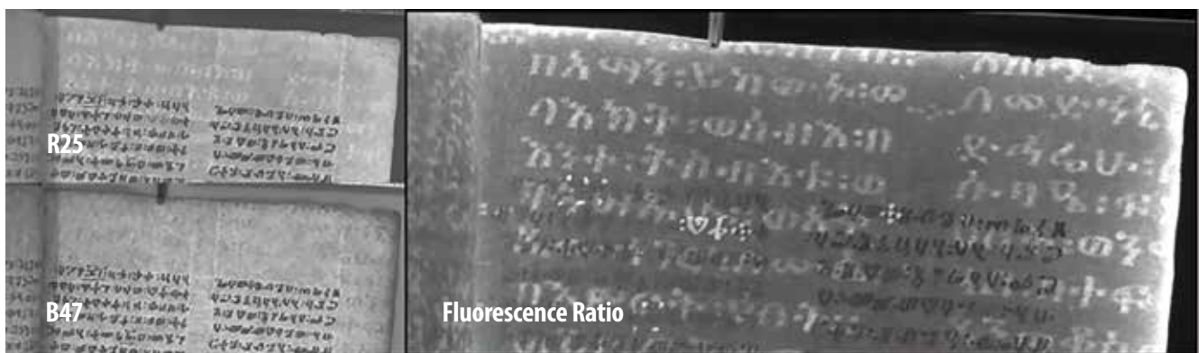
Fig. 8: By dividing the red-filtered image (R25) by the blue-filtered image (B47), the erased characters are significantly enhanced in the ratio image, shown on the right.
