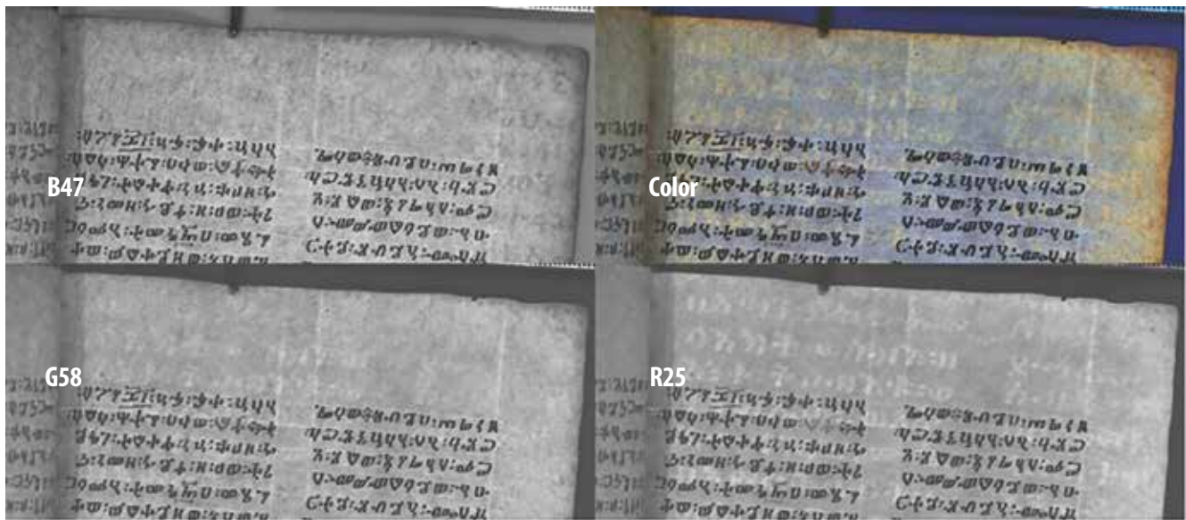
Fig. 7: The fluorescence of the erased text is different through the three color filters, B47 (blue), G58 (green) and R25 (red). The color fluorescence image is made from the three filtered-images.
