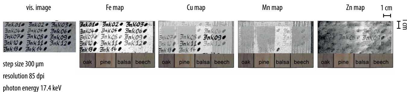
Fig. 6: Testing the method using iron-gall ink writing on modern thick parchment which was put face down onto different types of wood. The results show that the iron and copper maps are quite readable in all cases. The manganese and zinc maps from this test are rather illegible, with the zinc mostly showing the signal from the modern parchment rather than from the structure of the wood.
