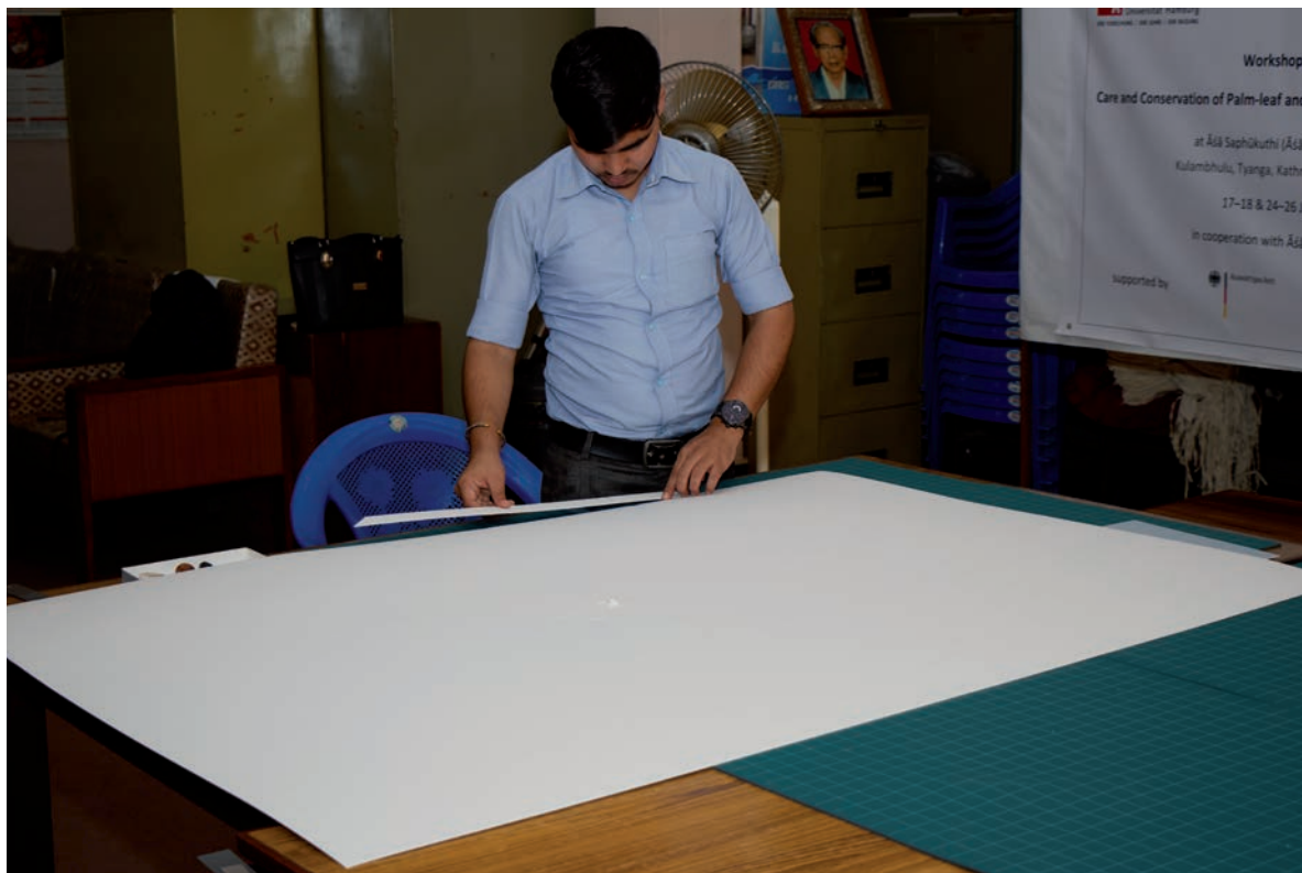
Fig. 25: The machinist square is used to verify that the bottom left corner of the E-Flute board is a 90-degree square. This corner is marked in pencil with a small square at the bottom left corner of the E-Flute board (Supplement, page 1). Measurements are now transferred onto the E-Flute used for the phase box using the measurement stick and board thickness jig (Supplement, page 1 – Construct a measuring jig) according to the formula shown in Biddle 2019.
