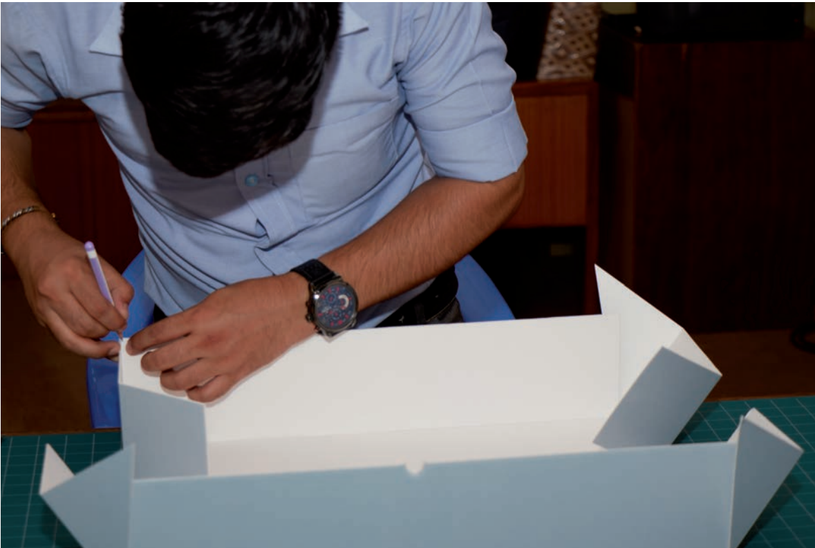
Fig. 39: The corners are checked to make sure all sides are equal. Should that not be the case, they must be trimmed. This has to be done before gluing as once the corners are glued it is almost impossible to trim the corners smoothly. Smooth cuts are important as paper whiskers will hold dust, can catch and tear.
