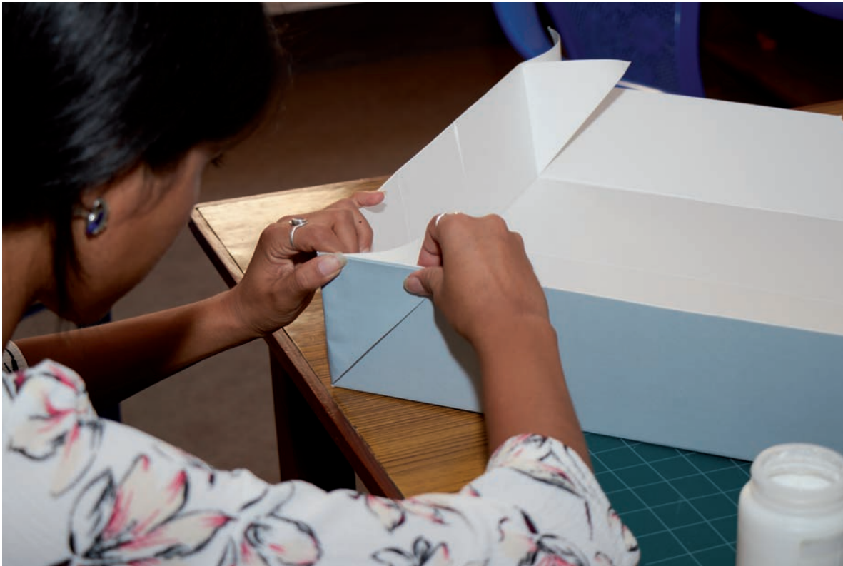
Fig. 43: The outer corner flap is connected to the outer board side after gluing.
