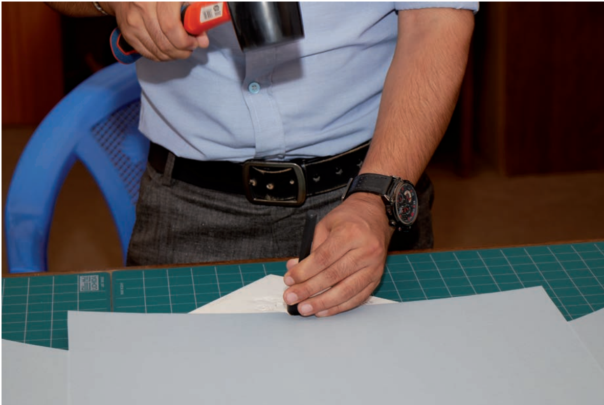
Fig. 35: A thumbhole (half-circle) is punched on the cover tray using a punch and fiberglass handled rubber mallet. As one is striking metal, it is important to use a rubber mallet in order to avoid a dangerous spark. Making a thumb hole arc helps to open the box easily as these boxes are very tightly fitted. The thumb hole arc should be made in the centre edge of the cover tray.
