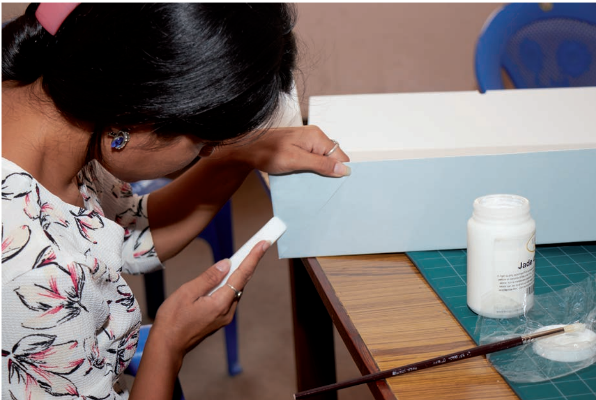
Fig. 44: The corner flap adhesion is increased, and wrinkles are smoothed out using a Teflon folder. The same process is applied for all four corners.
