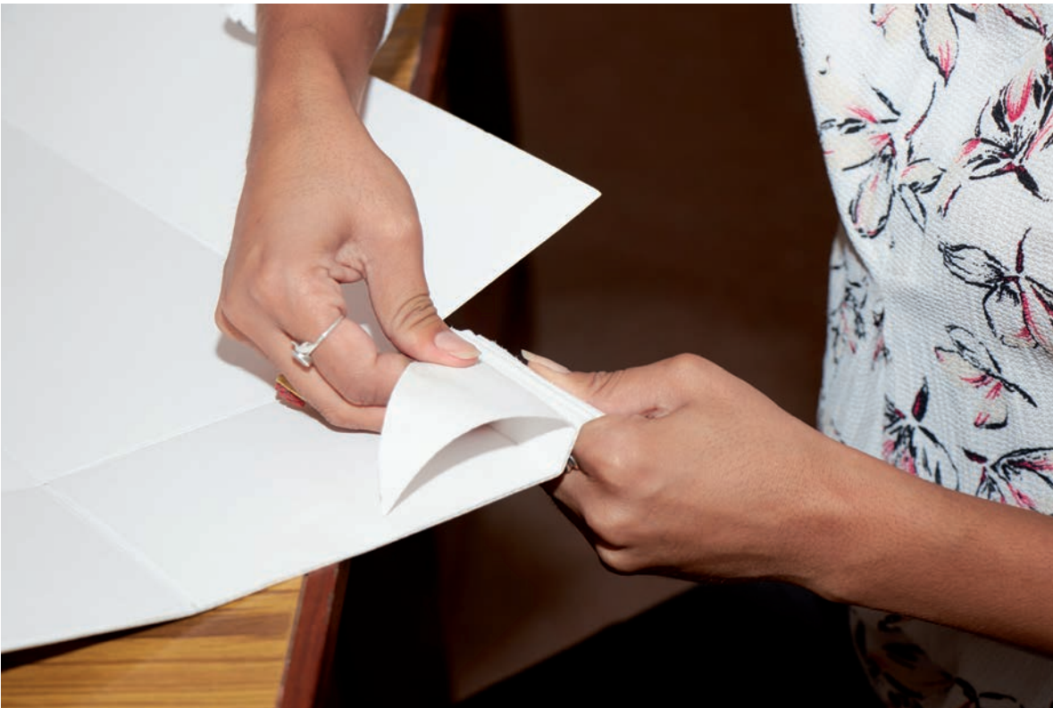
Fig. 40: The layers of the E-flute corner are separated.
