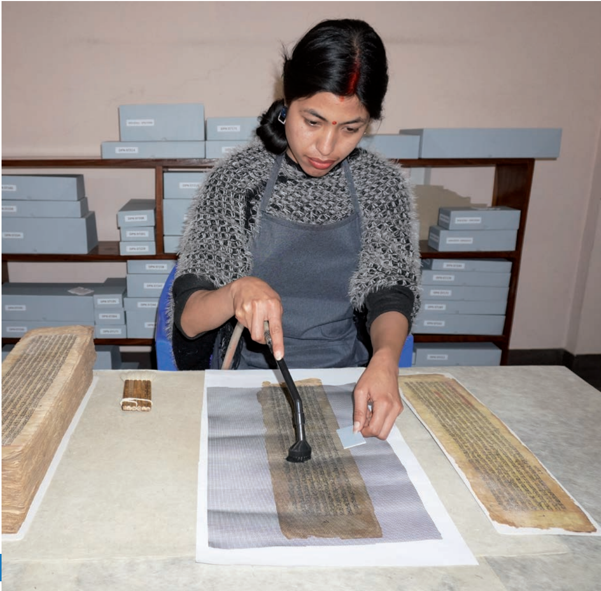
Fig. 4: The manuscript folio is cleaned using the variable speed-control HEPA vacuum with micro tools. A piece of polyester screening is placed on top of the folio during vacuum cleaning to prevent damaging the folio, or in case it has brittle sections or parts that are coming loose. The suction level is set very low and the folio is cleaned through polyester screening in order to ensure that brittle or loose edges are not pulled into the vacuum.
