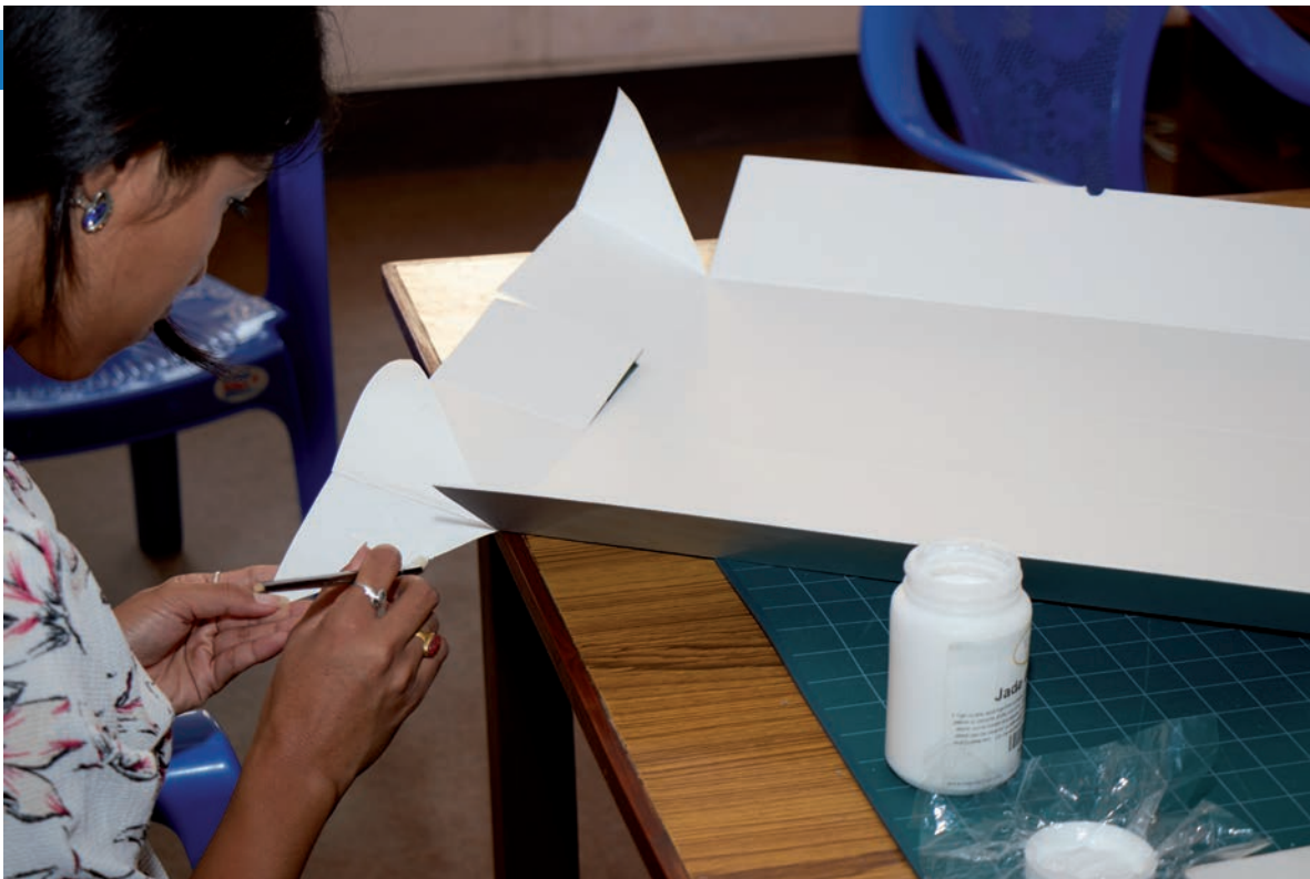
Fig. 42: The PVA Jade 403 is applied on the inner sides of the corner outer layers. Jade 403 is an acid-free, permanent adhesive that dries clear, mat and does not yellow over time.
