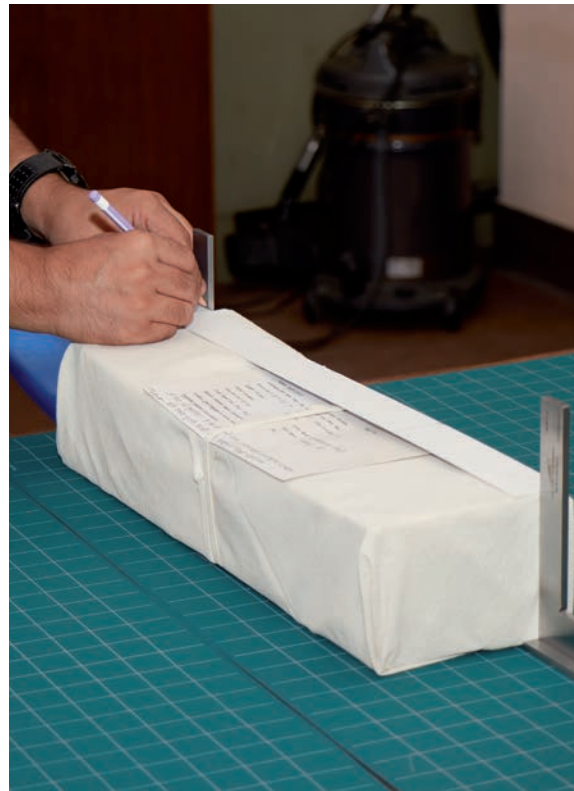
Fig. 21: The height (H) is measured. This measurement is repeated at three points along the short side.
