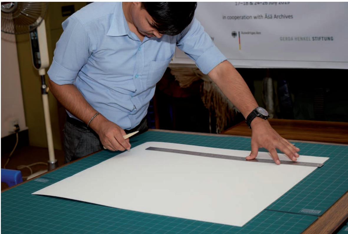
Fig. 27: The first vertical score line is now marked using the (tapered) bone folder. This is creating the front wall of the box cover (Supplement, page 1). Here one has to press the bone folder in a manner that produces a score line but without tearing the E-Flute board or making unnecessary holes.
