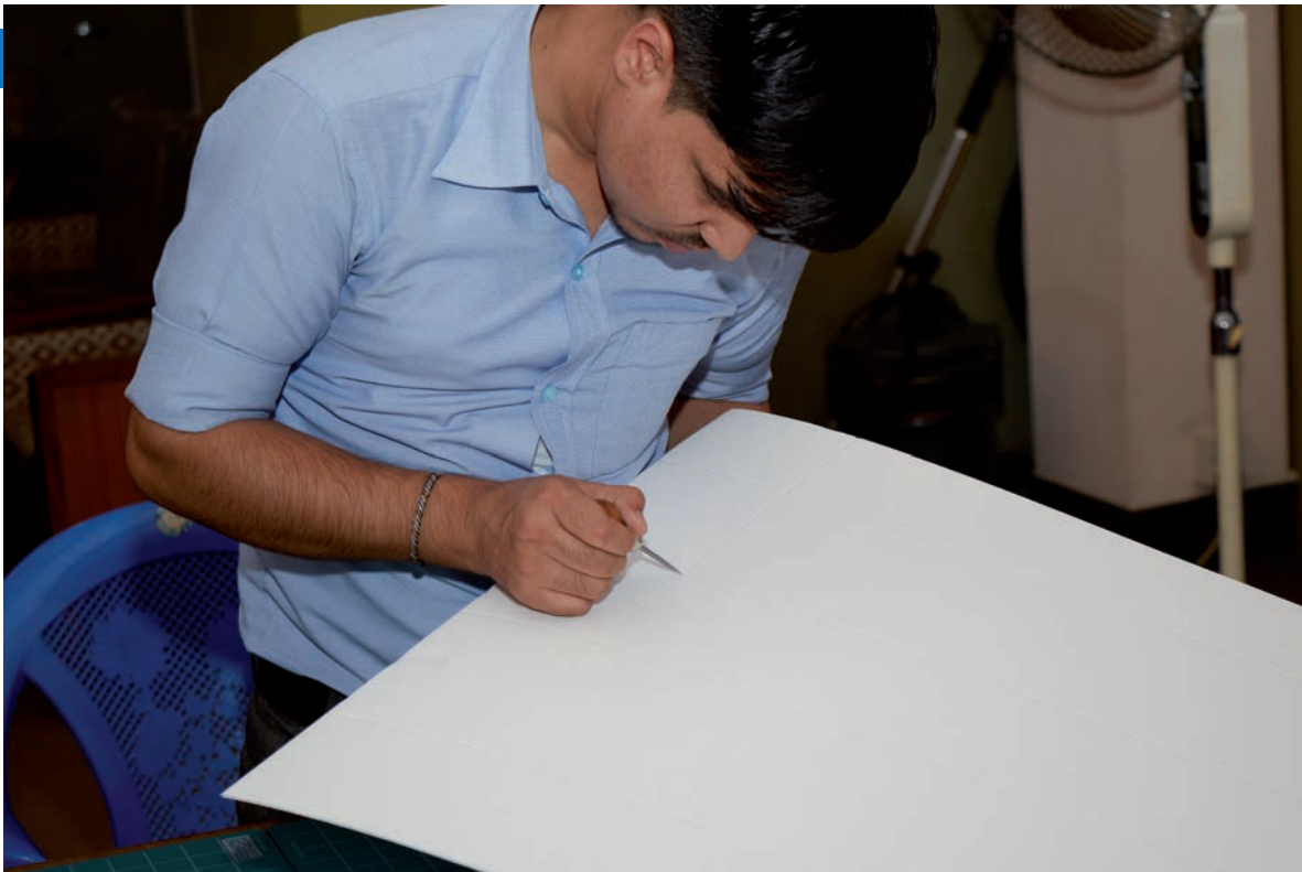
Fig. 30: After all lines have been made, a needle awl is used to mark the central point at the corner. Marking a small hole with the awl makes it easier to cut the downside of the cover tray and middle part of the bottom of the wall which, upon completion, will bend inwards while closing the box.
