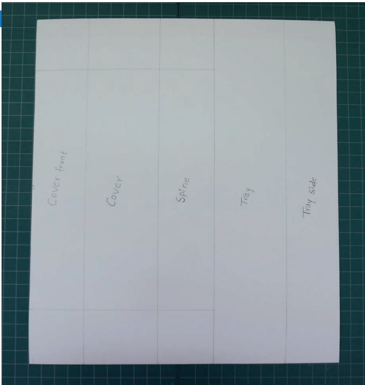
Fig. 26: Measurements are transferred onto the E-Flute using the measurement stick, the board thickness jig and a straight edge after the measurements made along the bottom and left side of the board are transferred to the top and middle side of the E-Flute (Supplement, steps 5 & 6).
