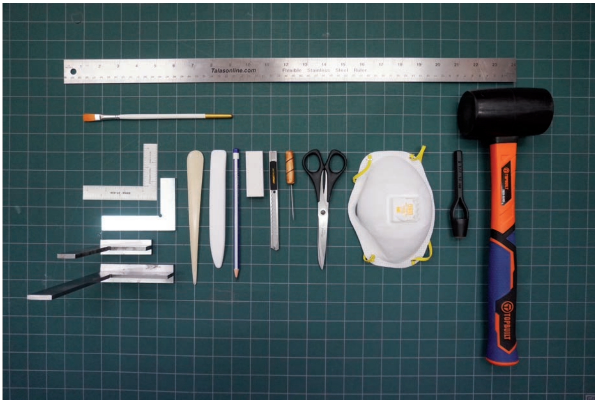
Fig. 6: Tools – (clockwise from lower left) – standing steel squares, flat machinist square, mini Zona square, brush, straight edge (ruler) with cork back, rubber mallet, 1 cm punch, N95 mask (especially for cleaning), shears, needle awl, Olfa silver breakaway knife, white rubber, graphite pencil, large Teflon folder, tapered bone folder
