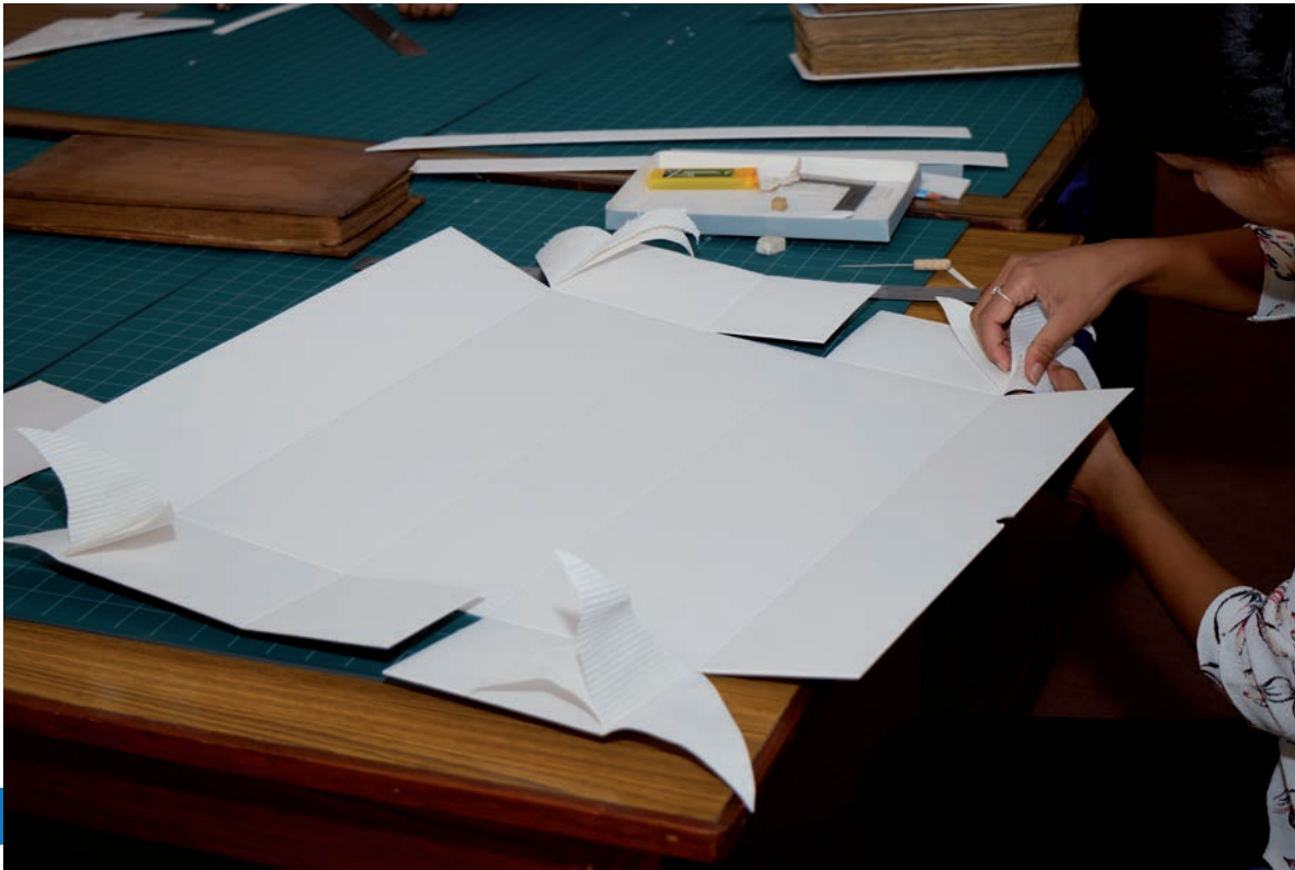
Fig. 41: When separating the layers of the E-flute corners, it is necessary to trim away the middle-corrugated material (Supplement, step 9) in order to ensure proper gluing which is key in creating the phase box's sturdiness.
