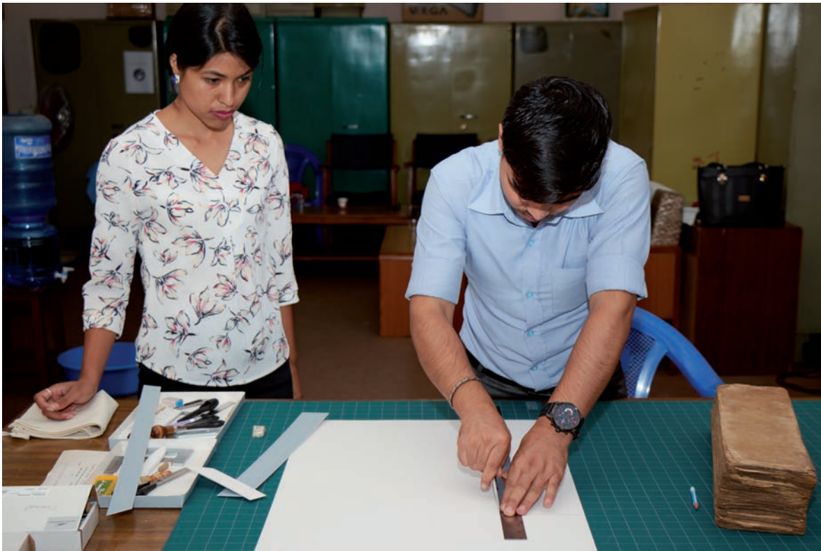
Fig. 10: The first cover board is cut out. A flexible stainless-steel straight edge (ruler) with an anti-slip cork backing is used to give the best support ensuring the cover is cut smoothly and accurately using an Olfa silver breakaway knife.
