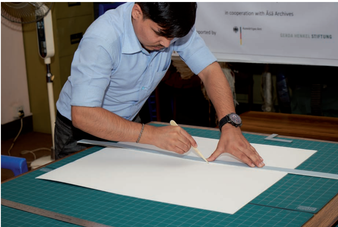
Fig. 28: The second vertical line is now made using the bone folder. The third and fourth vertical lines are also marked using the bone folder. The section between the second and third line will form the box wall between the cover and the tray. The section between the third and fourth line will form the base tray and the section between the fourth line and the right edge of the E-Flute board will become the wall of the box base tray.
