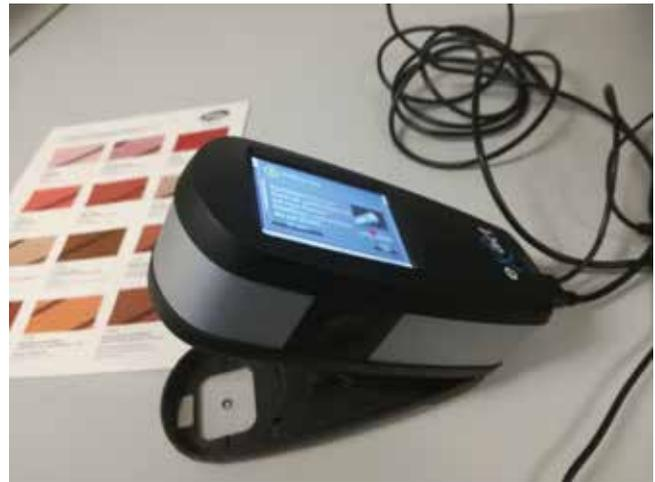
Fig. 2.2-5: VIS-Spektrometer X-rite exact, Messungen am Centre for the Study of Manuscript Cultures. | VIS spectrometer X-rite exact, used in measurements at the Centre for the Study of Manuscript Cultures.
